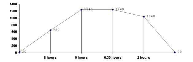
For this program illustrated in this graph, in step 1 the temperature goes: in 8 hours to 650 °C then to step 2: in 0 hours to 1240 °C which in step 3 we: switch for 30 minutes and in the cool-down phase step 4: in 2 hours to 1080 °C
